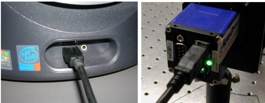
**Figure 7. Connect the AgilEye HWS camera to your computer via a USB cable.**
