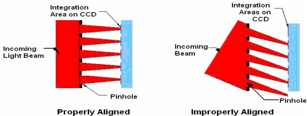
**Figure 4. Proper alignment of a Hartmann WFS**
