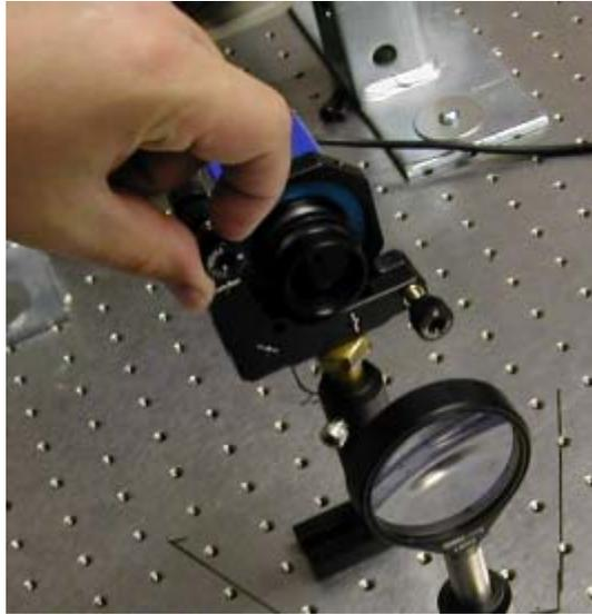
Figure 10. Adjust the tip-tilt mount on the AgilEye HWA...
