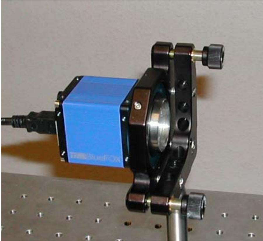
**Figure 2. AgilEye Shack-Hartmann Wavefront Sensor**
