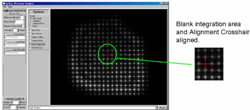
Figure 11. . . until the Alignment Crosshair is centered on the blank integration area.
