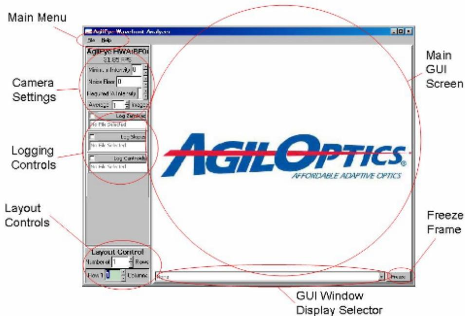
**Figure 23. AgilEye Main GUI Controls**
