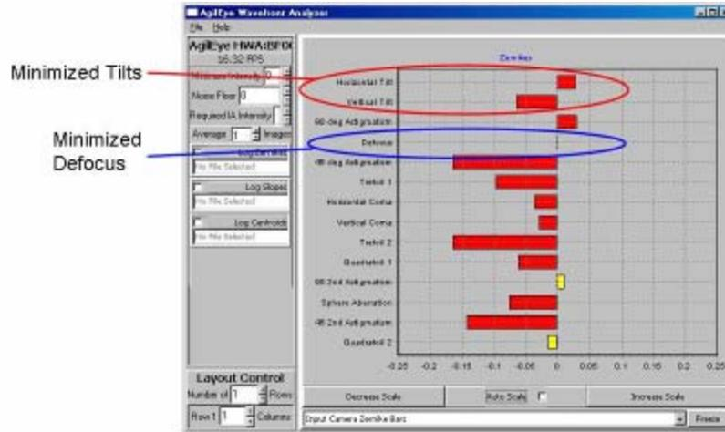
**Figure 13. Minimized X-Tilt, Y-Tilt, and Defocus**
