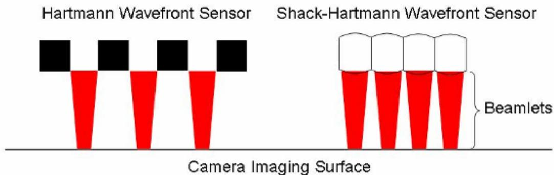
**Figure 5. Hartmann and Shack-Hartmann imaging wavefronts**
