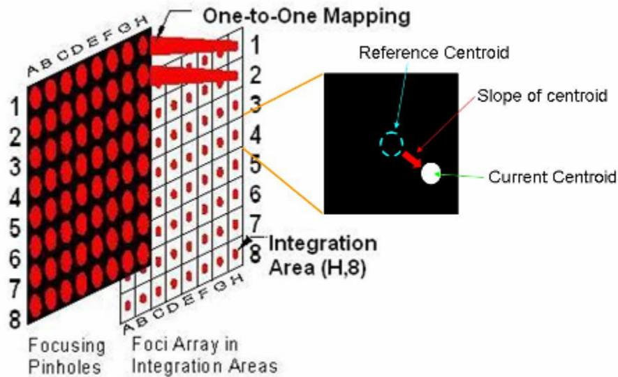
**Figure 3. Pin hole integration areas of a Hartmann Wavefront Sensor**
