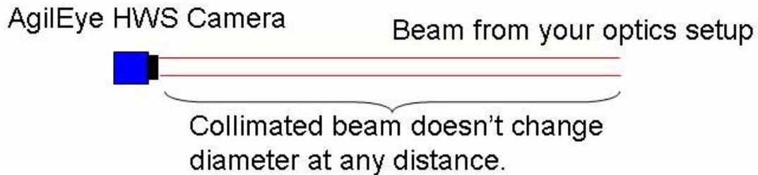
**Figure 6. Collimated input beam for AgilEye**
