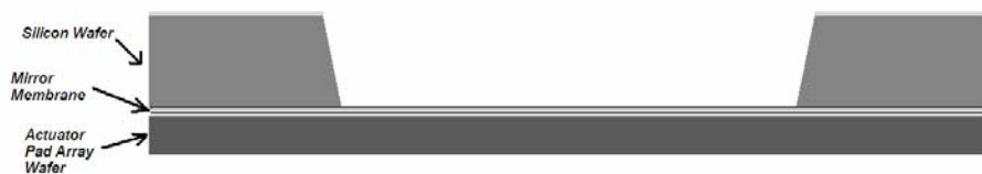
Diagram of a Deformable Mirror
