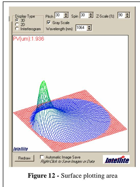
Figure 12 - Surface plotting area
