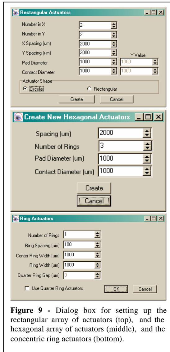
**Figure 9** - Dialog box for setting up the rectangular array of actuators (top), and the hexagonal array of actuators (middle), and the concentric ring actuators (bottom).
