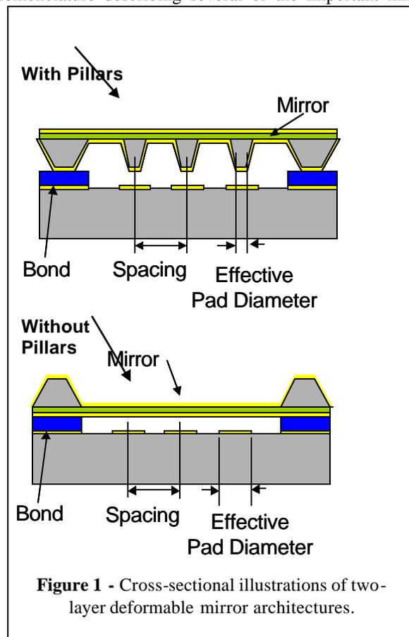
**Figure 1** - Cross-sectional illustrations of two-layer deformable mirror architectures.
