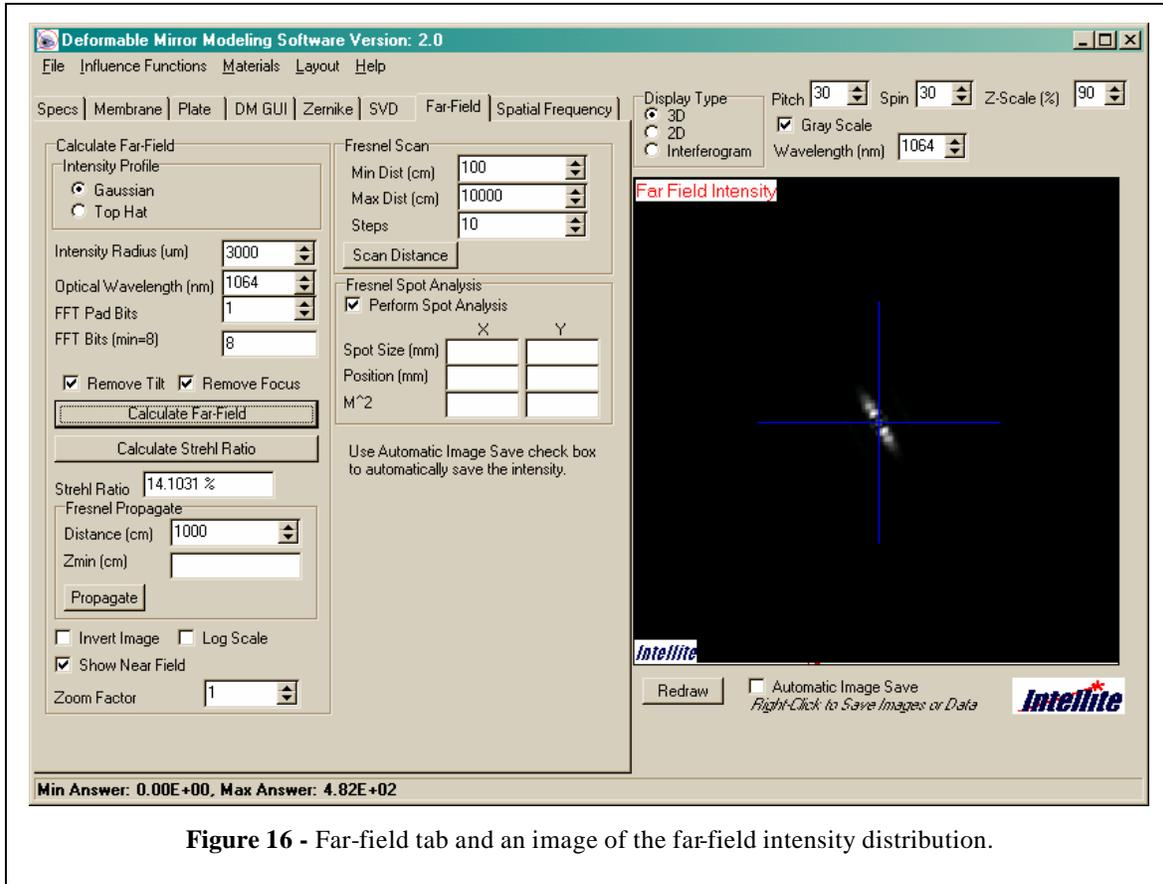
Figure 16 - Far-field tab and an image of the far-field intensity distribution.
