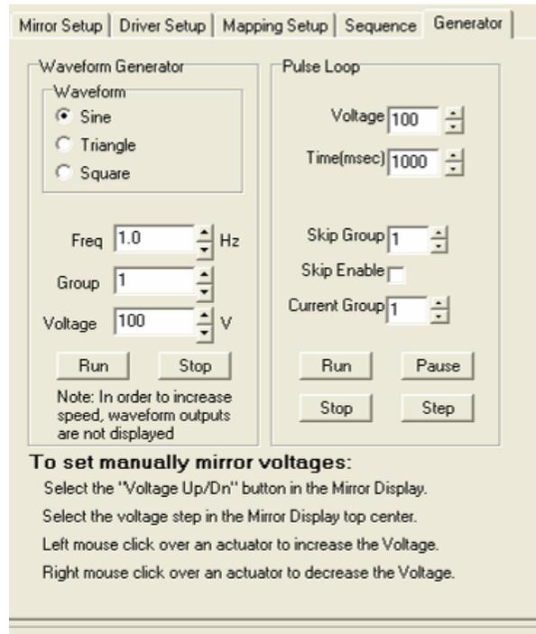
Figure 18: Generator Tab
