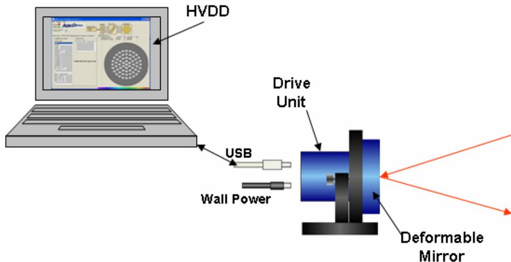
**Figure 1: Functional Block Diagram of HVDD in Operation**
