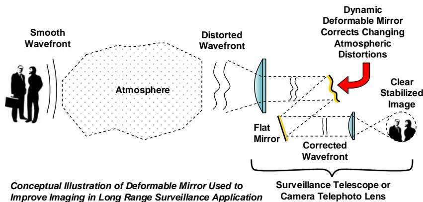
Figure 4: Atmospheric Aberration Correction
