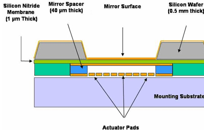
Figure 3: Cross section of an AgilOptics' Deformable Mirror
