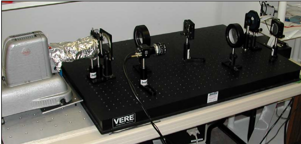
Figure 9 Photograph of setup for testing Image Sharpness
